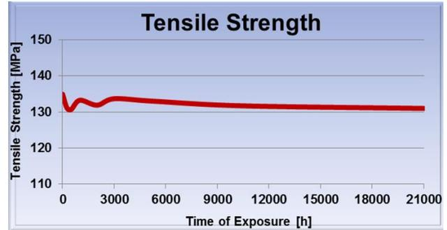
Figure 2: Tensile strength retention under accelerated Xenon-arc UV weathering of glass fiber reinforced Ultradur<sup>®</sup>
