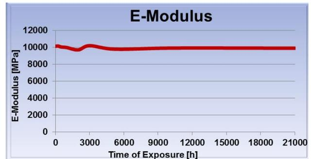
Figure 3: Tensile modulus property retention under accelerated Xenon-arc UV weathering of glass fiber reinforced Ultradur<sup>®</sup>
