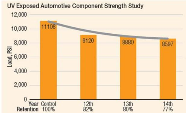
Figure.1: Tensile strength retention over years of service. Actual UV exposed glass fiber reinforced Ultramid<sup>®</sup> automotive component.
